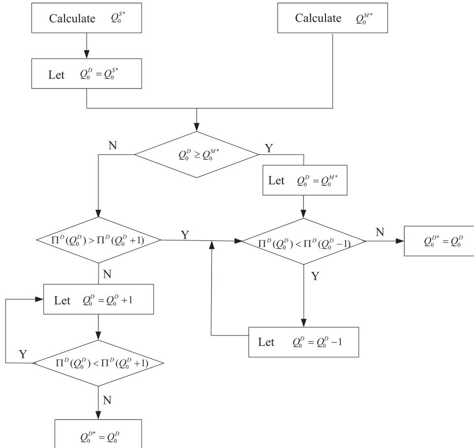
**Fig. 5.** Algorithm for the dynamic allocation policy.
